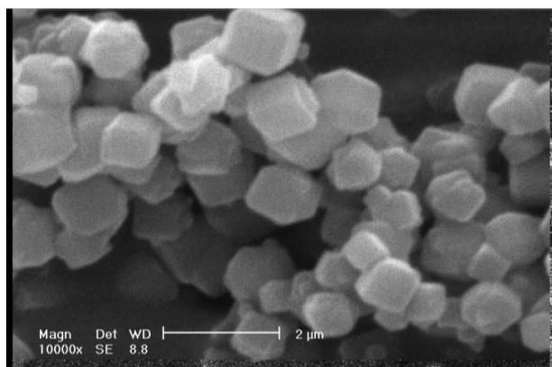
**Figure 3. SEM image of LTA zeolite.**
