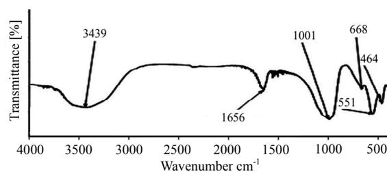
Figure 1. FTIR spectra of LTA zeolite.
