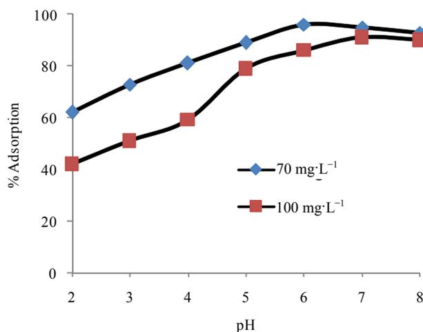
**Figure 4. Effect of pH on the adsorption of Fe(III) onto LTA zeolite.**
