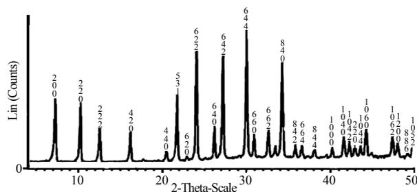
Figure 2. XRD pattern of LTA zeolite.
