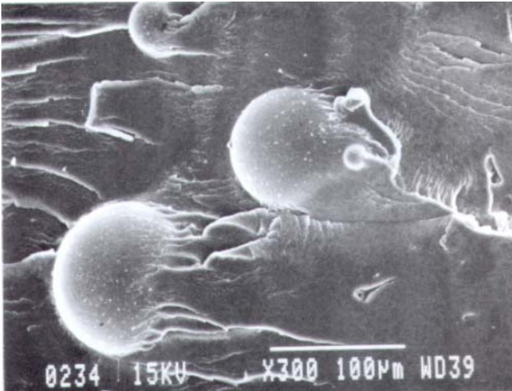
Figure 6. SEM photograph of fracture surface of LDPE/GB2227 composite.
