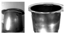
Figure 4. Blanks with Cracks.
