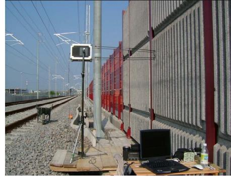
**Figure 2.** Reflection index measurement according to CEN/TS 1793-5 along a railway line.
