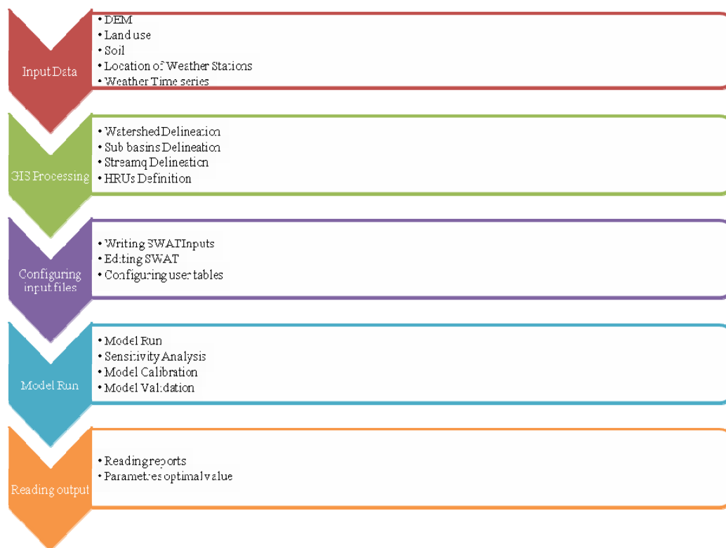
Figure 3. Components and input/output data of SWAT model.
