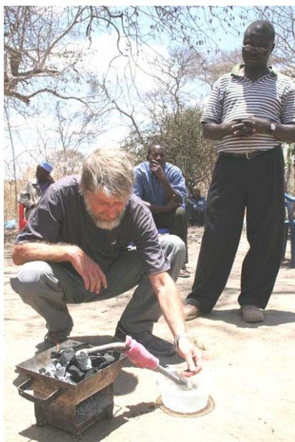
Figure 2. Retort for distillation of mercury.
