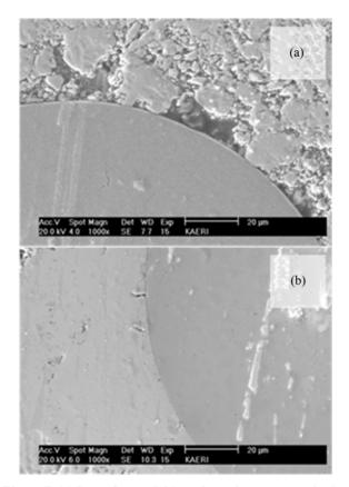
Figure 7. (a) Imperfect and (b) perfect microstructure in the interface between Zr matrix and ZrO<sub>2</sub>. SEM image of polished surface.
