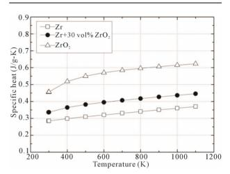
Figure 5. Calculated specific heat of simulated fuel.
