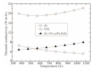
Figure 8. Comparison of thermal conductivity of Zr,  $UO_2$  and  $ZrO_2$ -Zr simulated inert matrix fuel.
