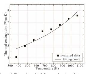
Figure 6. Thermal conductivity as a function of temperature of simulated inert matrix fuel based on the measured and calculated data.
