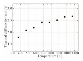
Figure 3. Measured thermal diffusivity as a function of temperature of simulated inert matrix fuel.
