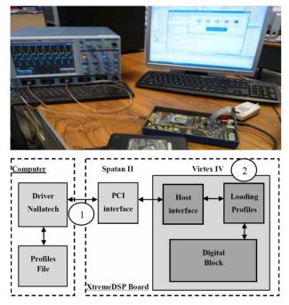
Figure 5. Connection between the computer and the XtremeDSP board.
