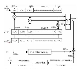
Figure 4. FIR 147 with 23 multipliers for one  $h_{11}$  and  $h_{21}$ .
