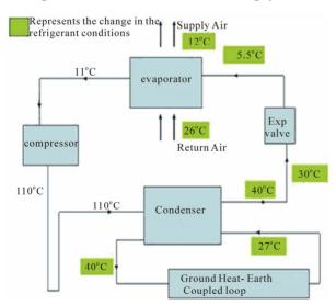
Figure 3. An earth coupled geoexchange system.
