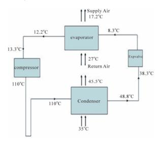
Figure 2. A conventional air conditioning system.
