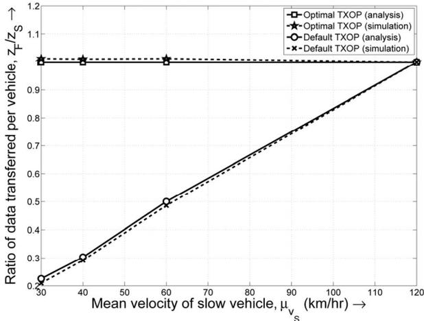
Figure 4. Ratio of data transferred per node vs velocity of slow vehicle with default scheme and TXOP tuning ( $\mu_{v_F} = 120$  km/hr,  $\sigma_{v_S} = \sigma_{v_F} = 5$  km/hr).
