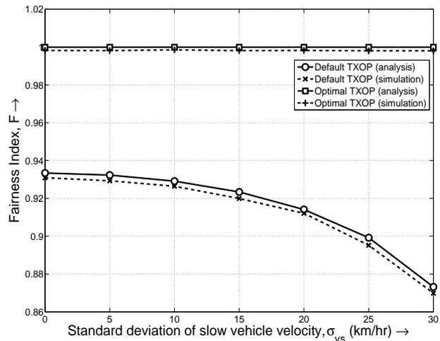
**Figure 6. Fairness index vs standard deviation of slow vehicle speed ( $\mu_{v_S} = 60$  km/hr,  $\mu_{v_F} = 120$  km/hr,  $\sigma_{v_F} = 5$  km/hr).**
