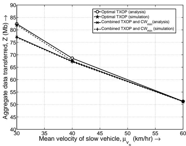
**Figure 8.** Aggregate data transferred vs mean velocity of slow station ( $\mu_{v_F} = 120$  km/hr and  $k_{jam} = 80$ ,  $\sigma_{v_s} = \sigma_{v_F} = 5$  km/hr).
