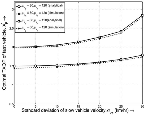
**Figure 5. TXOP of fast vehicle vs standard deviation of slow vehicle speed ( $\sigma_{v_F} = 5$  km/hr).**
