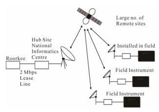
Figure 4. A diagram showing the networking of instruments installed in field to Roorkee (the central station).
