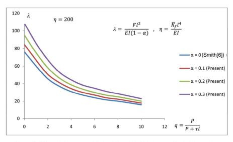
Figure 5. Effect of damage on pile buckling with 200% normalised soil modulus.
