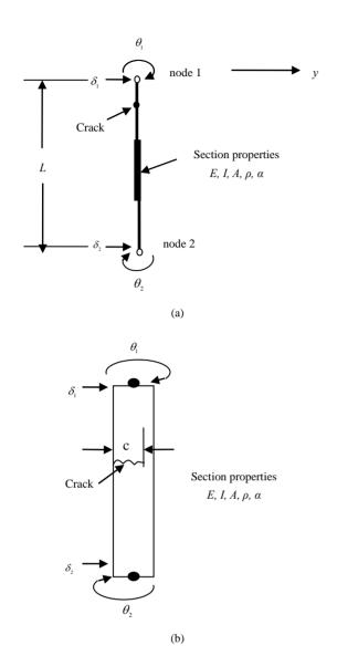
Figure 1. (a) Typical discrete flexural line element; (b) Enlarged details of cracked element
