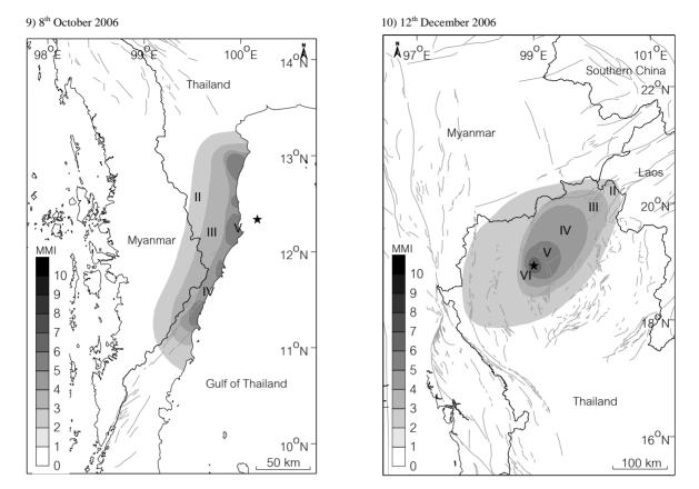
**Figure 1.** Isoseismal maps of the ten earthquakes reported in Myanmar and neighboring areas during 1912-2006 AD. Grey thin lines illustrate the earthquake faults based on Bender *et al.* [6] and Pailoplee *et al.* [4]. Black stars are the locations of past earthquakes whereas the ground shaking intensities are illustrated in terms of gradual color of the MMI scale.
