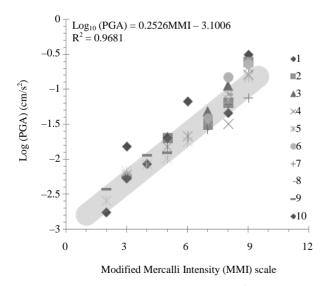
**Figure 2.** Relationship between the PGA  $(cm/s^2)$  and the MMI scale. The series of MMI-PGA data are distinguished by different symbols and the numbers correspond to the isoseismal maps in **Figure 1**. The correlation coefficient ( $R^2$ ) for the shown linear regression is 0.9681.
