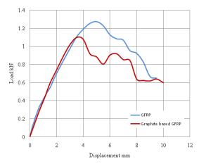
Figure 7 Typical force-deflection curves from the ENF specimens
