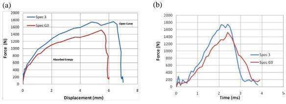
Figure 10 Typical graphs of the laminate for impact velocity of 4.429 m/sec
