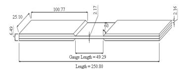
Figure 1 Dimensions of tensile test specimen
