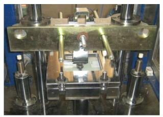
Figure 5 Specimen clamping apparatus
