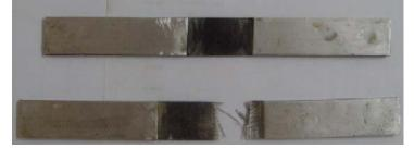
Figure 2 Tensile test specimens before and after tensile testing
