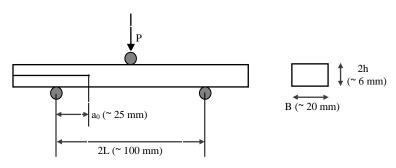
Figure 4 Schematic diagrams of the set-up for ENF test
