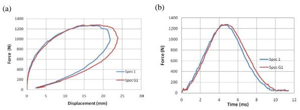
Figure 8 Typical graphs of the laminate for impact velocity of 2.215 m/sec
