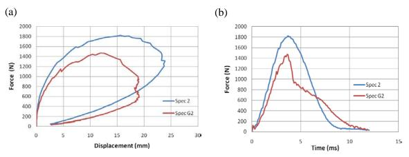
Figure 9 Typical graphs of the laminate for impact velocity of 3.132 m/sec
