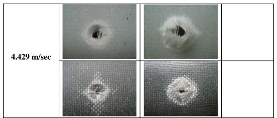
Figure 11 Post-perforation images of damaged specimens
