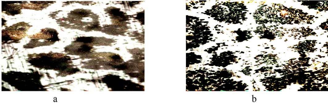
Plate 3 Microstructure of as-cast sample (**A**-  $\alpha$ -aluminum, **B**-  $Mg_2Si$ ).
