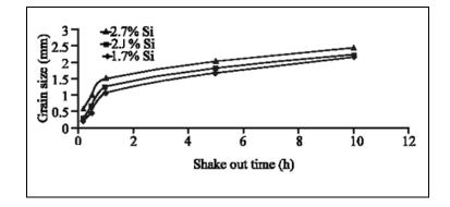
Fig.2: Plot of effect of shake-out time on grain size
