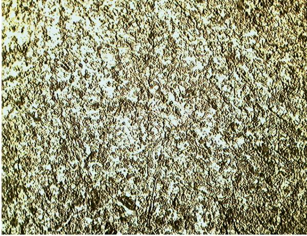
Fig 12: Micrograph of as-cast Al-6%Zn showing  $\alpha$ -Al matrix(white) and  $\beta$ -Zn phase dark. 200X
