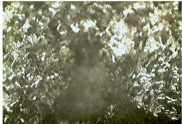
Fig 11: Micrograph of Al-4%Zn after immersion in seawater for 8 weeks showing dark regions of corrosion product. 200X
