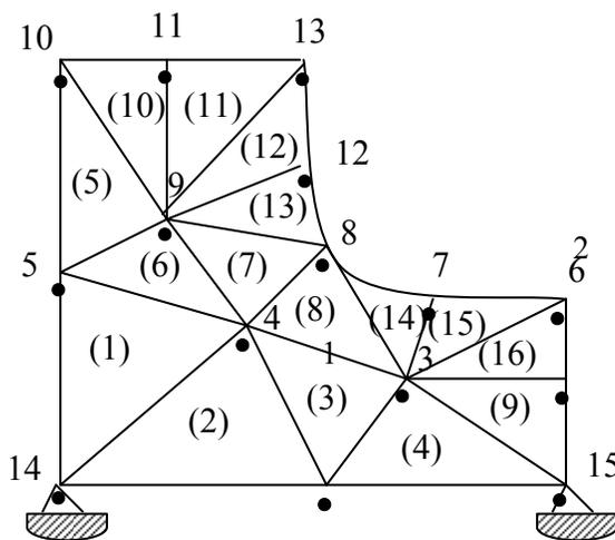
Figure 1: Idealized Finite element Model of two Dimensional Composite Body.
