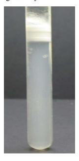
Figure-1 Growth of CaSeHPO<sub>4</sub> crystals at laboratory environment
