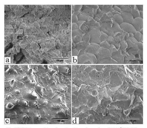
Fig. 2 SEM images taken from the sintered samples. a)  $1000^{\circ}C \times 20$  min; b)  $1050^{\circ}C \times 20$  min; c)  $1100^{\circ}C$  without holding time; d)  $1075^{\circ}C$  without holding time
