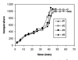
Fig.1 Tempeture profile for mw sintering of Mg<sub>2</sub>F
