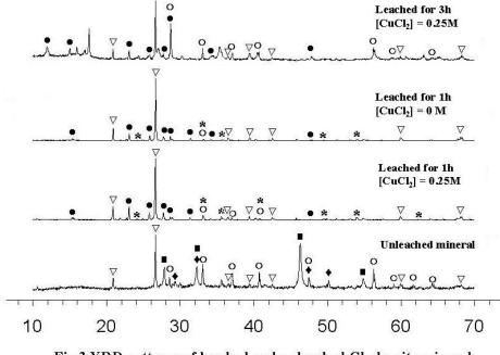
Fig.3 XRD patterns of leached and unleached Chalcocite minerals ● Sulfur, ◆ Spionkoptite, ■ CuFeS<sub>5</sub>, ○ Pyrite, \* Hematite ⊽ Quartz.
