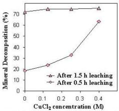
Fig.5 Effect of weighed-in CuCl<sub>2</sub> concentratration on the leaching. Leaching conditions: 135°C, 45psi oxygen pressure, 0.4M NaCl, 100g/l mineral and the HCl concentration varied with the CuCl<sub>2</sub> to keep a constant [Cl<sup>-</sup>] of 1.9M.
