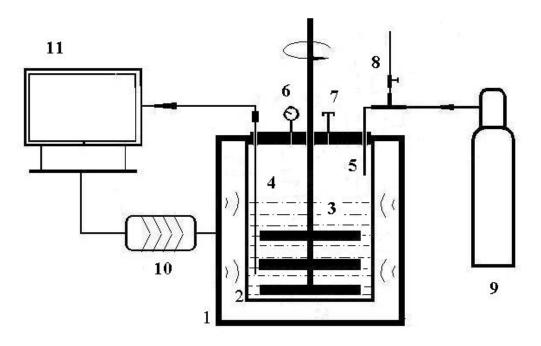
Fig.1 Microwave-hydrothermal reactor used for chloride leaching of copper sulfide minerals under oxygen pressure
