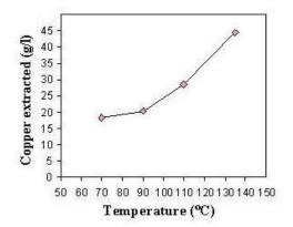
Fig.4 Effect of temperature on leaching Chalcocite: 100g/l; CuCl<sub>2</sub>:0.25M; NaCl: 0.4M; HCl: 1.0M; leaching time: 2hours
