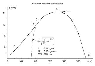
Figure 5. The measured angular velocities from forearm rotation downwards (points on the curve A-E) and the theoretical angular velocity values calculated from Equation 15 (broken line). The zero point of time for the theoretical angular velocity curve is at the intersection of the time-axis and the broken-line curve (the same time scaling is same for both curves).
