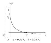
Figure 1. Hill's equation  $(F + a)(v + b) = b(F_0 + a)$  where  $F_0$  is so-called isometric force or force with zero velocity,  $v_0$  is the highest possible velocity, a and b are constant force and constant velocity. In rotational movement torque M corresponds to force F and angular velocity  $\varphi$  corresponds to velocity v.
