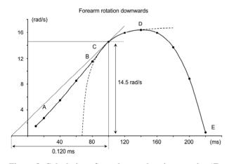
Figure 8. Calculation of angular acceleration at point (T = 0.10 s,  $\dot{\varphi} = 14.5$  rad/s), where the theoretical angular velocity curve (broken line) coincides with the measured angular velocity curve (points) between C-D.
