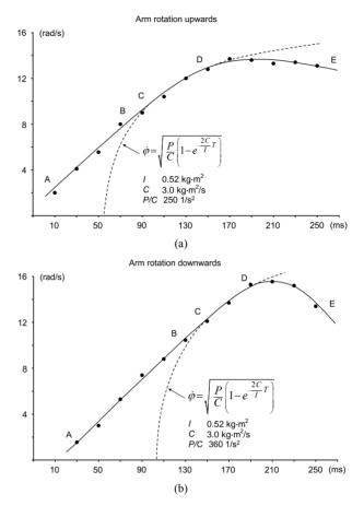
Figure 7. The measured angular velocities (points on the curve fitting A-E) from the whole arm rotation downwards (a) and upwards (b) and the theoretical angular velocity values calculated from Equation 15 (broken lines). The zero point of time for the theoretical angular velocity curve is at the intersection of the time-axis and the broken-line curve.
