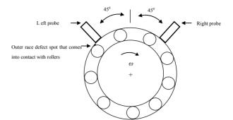
Figure 3. Probe orientations and outer race defect spot causing "ringing" of the bearing.
