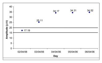
Figure 7(c). On-line imbalance of shaft defect for the 5 (NDEA) undamaged pump bearing.
