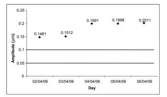
Figure 7(d). On-line misalignment of the shaft defect for the 3 (DEA) motor bearing.
