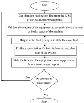
Figure 6. Process algorithm for fault diagnosis.
