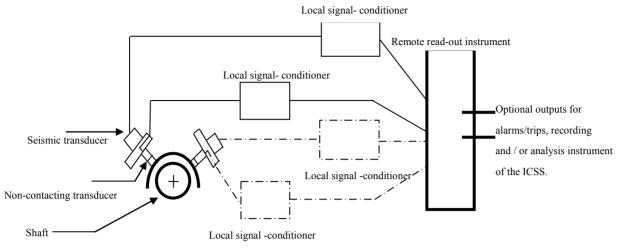
Figure 2. The probe arrangement.
