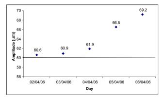
Figure 7(a). On-line displacement of shaft defect for the 5 (NDEA) pump bearing.
