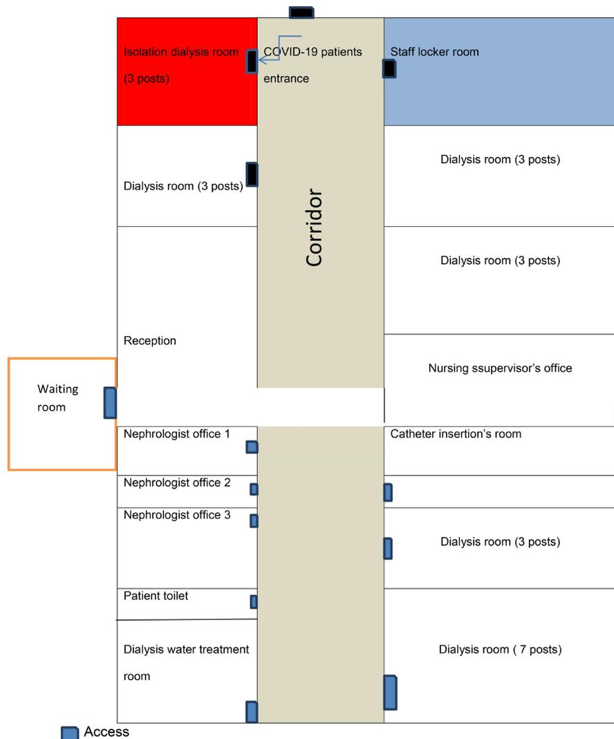
**Figure 1.** Plan of the hemodialysis unit.
