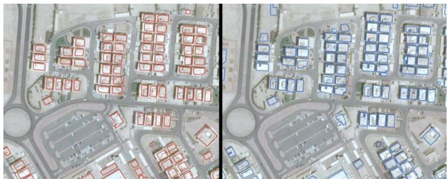
**Figure 7.** Building footprints digitized manually on the left compared to the deep learning algorithm outputs on the right.
