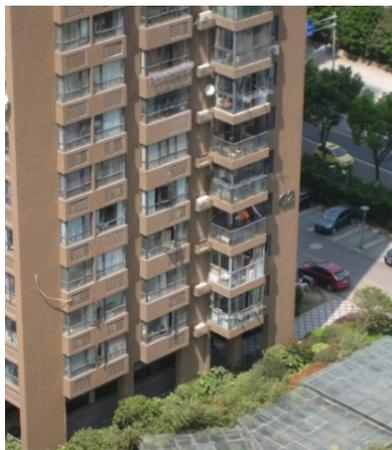
**Figure 5.** High-rise apartments, Ningbo block H: inappropriate climatic design with only a few of the apartments facing south and less opportunities for cross-ventilation, double-sided ventilation, and natural lighting (source: the authors).
