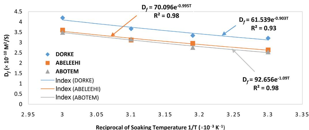
**Figure 3.** Relationship between diffusion coefficient ( $D_f$ ) and temperature ( $T$ ) for *Abotem Abeleehi* and *Dorke SR*.
