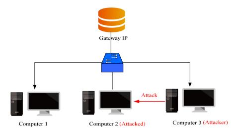
Figure 2. ARP (Address Resolution Protocol) spoofing topology diagram.
