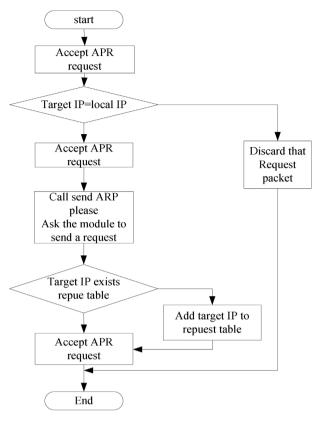
**Figure 3.** ARP (Address Resolution Protocol) request detection module.
