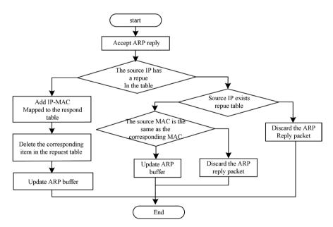
Figure 4. Flowchart of ARP (Address Resolution Protocol) reply packet detection algorithm.
