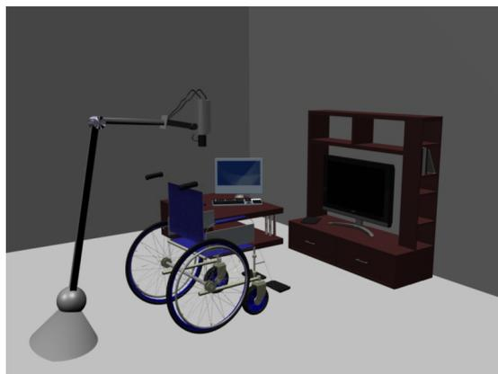
**Figure 2.** Structure of the prototype developed with the different parts: camera, user screen, and control PC related to the position of the user.
