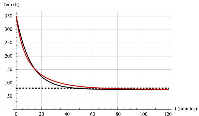
**Figure 2.** The solid red curve is the temperature profile of Model 2, Equation (5). The black curve is the profile of Model 1, Equation (2).
