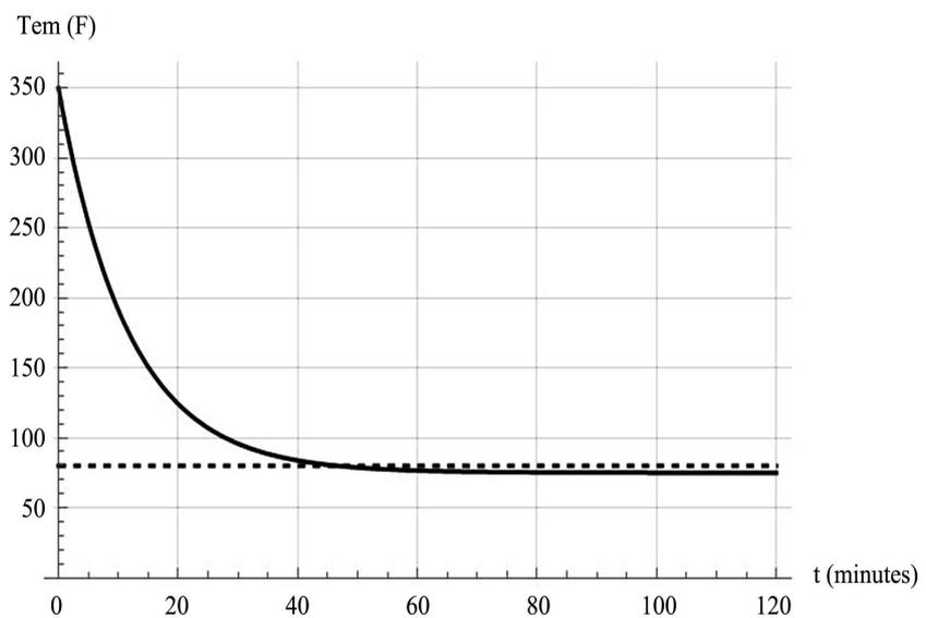
**Figure 1.** Plots of the temperature profile of cooling of the hot object (solid black), and the constant final aimed temperature (dashed black), respectively.
