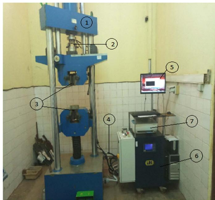
Presentation of the LaboGenie's compression-tension testing device: 1: Universal machine base; 2: Adapted bending test equipment; 3: Tensile-compression testing equipment; 4: Data cable; 5: Data reading interface; 6: Control unit; 7: Printer.
