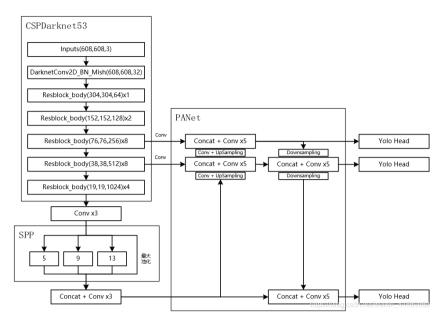
Figure 3. YOLOV4 network structure.
