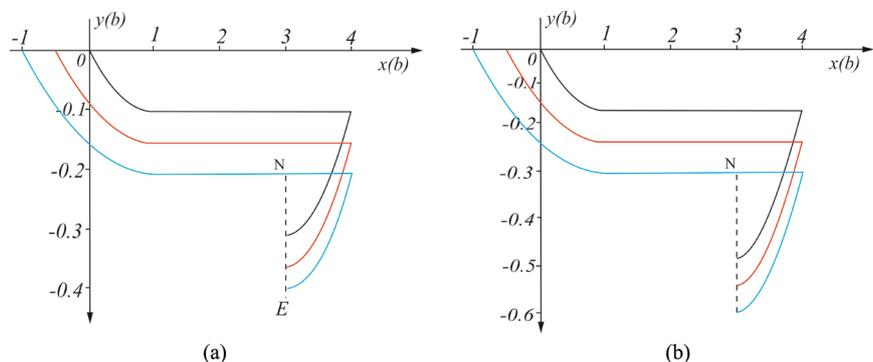
Figure 4. Airflow  $c = 0.2$  (a) and  $c = 0.4$  (b), obsesses  $x_0$  various value of the cotton slice effecting trajectories: 1—  $x_0 = 1$ , 2—  $x_0 = 0.5$ , 3—  $x_0 = 0$ .
