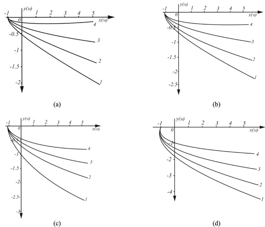
**Figure 2.** Speed air-influenced mainstream piece of pipe initial velocity [5].  $v_{0y} = 1$  m/c (a),  $v_{0y} = 2$  m/c (b) and  $v_{0y} = 3$  m/c (c) and (d) the value of the parameter  $\beta$  in various trajectories: 1—  $\beta = 1$ , 2—  $\beta = 1.2$ , 3—  $\beta = 1.5$ , 4—  $\beta = 2$ .
