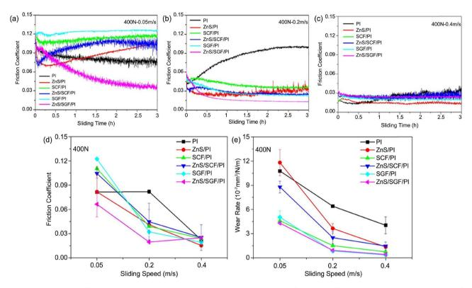
**Figure 6.** Friction coefficients against sliding time at various speeds (a-c); mean friction coefficients and wear rates (d and e) of PI-based materials against sliding speeds. Applied load: 400 N [76].
