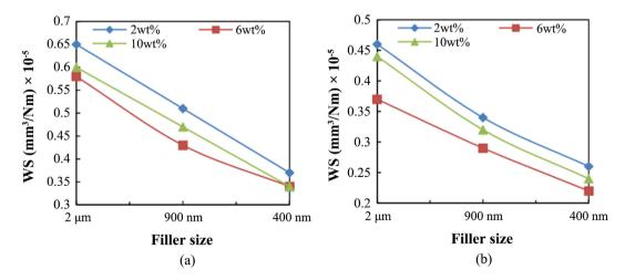
**Figure 3.** Variation of specific wear rate with filler size of (a) normal load applied, 10 N and 1.9 m/s and (b) normal load applied 70 N, and 5.7 m/s [40].
