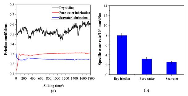
**Figure 5.** Coefficients of friction Variation (a) and specific wear rate (b) of PI/GO composites (load: 3 N, sliding speed: 0.1569 m/s, Duration: 30 min) [51].
