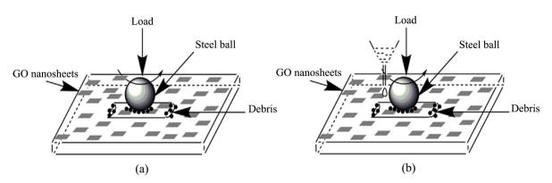
**Figure 4.** PI and PI/GO nanocomposites film for tribological applications (a) under dry friction and (b) under seawater lubrication [51].
