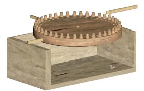
Figure 10. Peg wheel and drum with pebbles.
