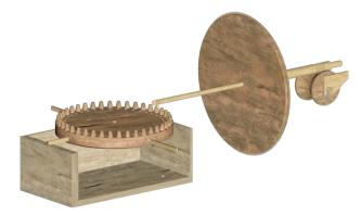
Figure 9. Longitudinal shaft and the two mileage counting systems.
