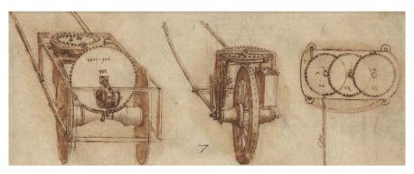
**Figure 6.** Design of the odometer by Leonardo da Vinci in folio 1r-b of the Codex Atlanticus.
