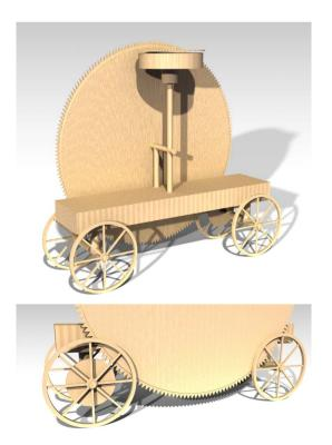
**Figure 3.** Reconstruction of Vitruvius' odometer according to Schofield (2016) (a 180 teeth gear is represented for sake of readability).
