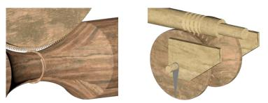
Figure 11. Use of the worm gear in the odometer of Leonardo da Vinci.
