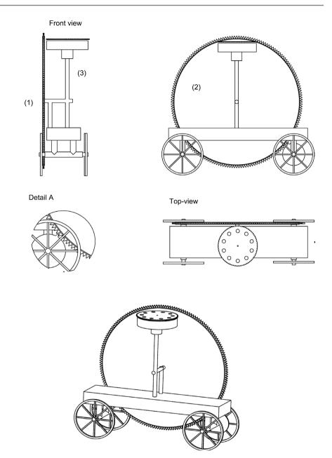
Figure 4. Sketch of Vitruvius' odometer (a 180 teeth gear is represented for sake of readability).
