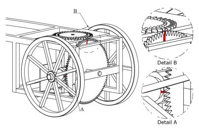
**Figure 5.** Reconstruction of Vitruvius' odometer according to Sleeswyk (1981) (a 100 teeth gear is represented for sake of readability).
