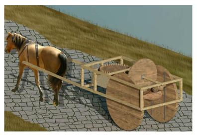
Figure 7. Digital reconstruction of Leonardo's odometer.
