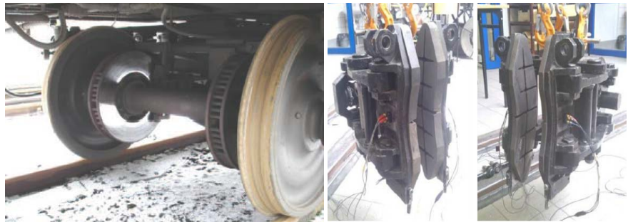
Figure 5. Eyeshots of the high speed axel mounted lining/disc brake unit.
