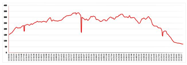
Figure 36. Surface temperature of the right pipe Thermocouple n°2. Aphelion.
