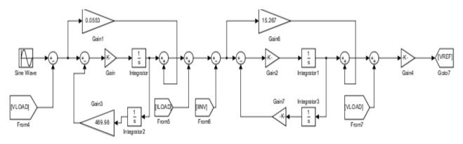
Figure 8. PR controller block in MATLAB.
