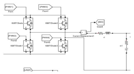
Figure 6. Inverter and LC filter in MATLAB.
