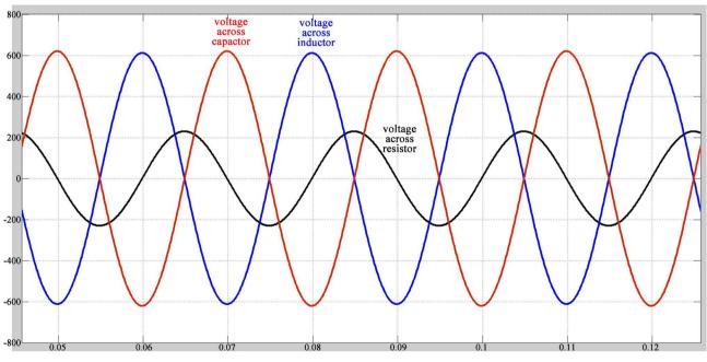
Figure 10. The simulation result for RLC Circuit (1.0 hp air-con).
