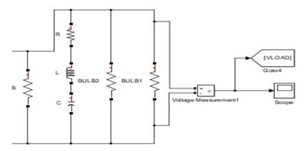
Figure 7. Load circuit with voltage sensor measurement.
