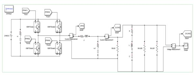
Figure 4. IGBT Inverter with load circuit only.
