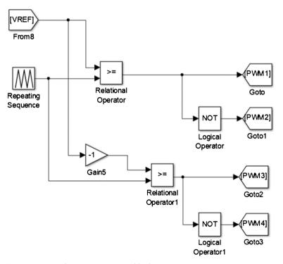
Figure 9. Unipolar PWM generator block.
