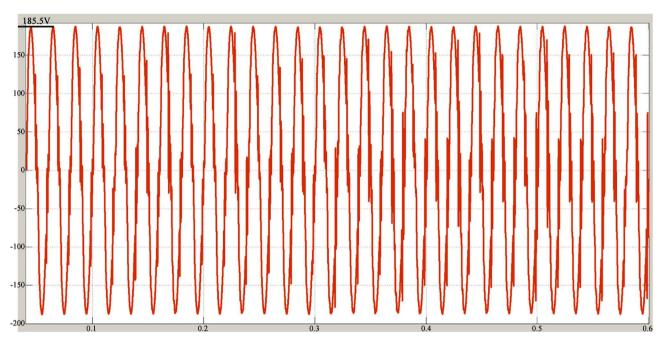
Figure 3. The waveform of the load output voltage for PR controller (inverter circuit only).
