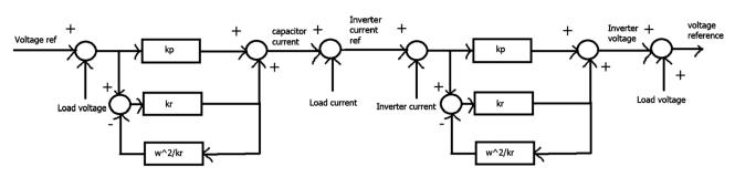
Figure 2. Block diagram for the PR controller.
