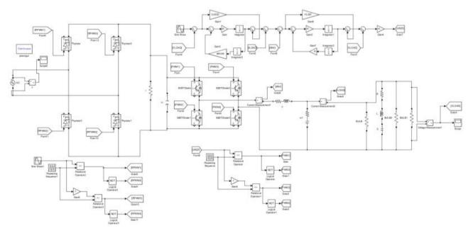
Figure 5. Energy-saving circuit with closed-loop PR controller.
