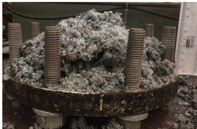
**Figure 21.** Debris obtained from experiment with M/W = 0.51.
