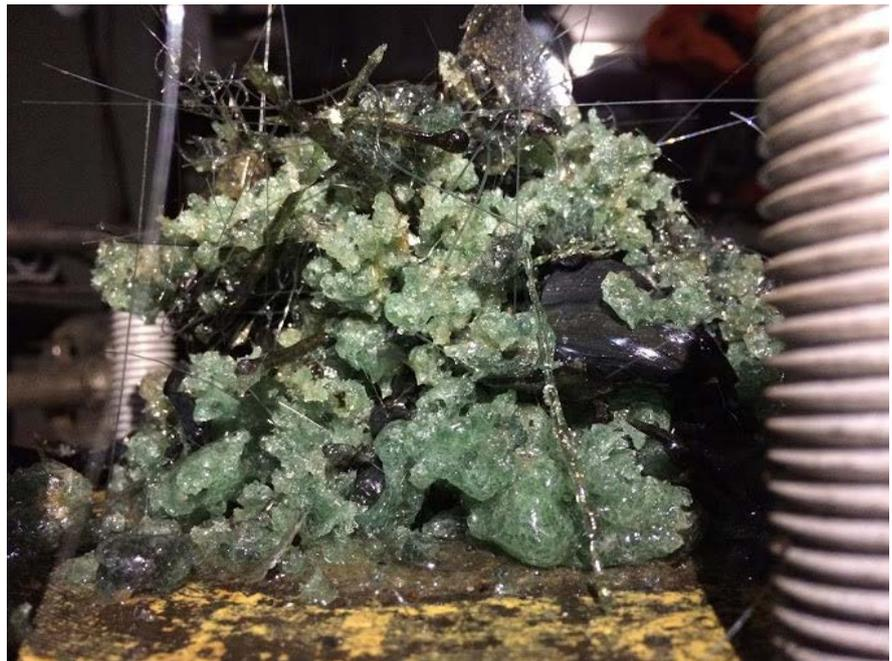
**Figure 14.** Debris obtained from experiment with M/W = 0.16.
