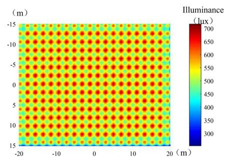
**Figure 5.** Illumination distribution map of agricultural greenhouse (experimental group experiment).
