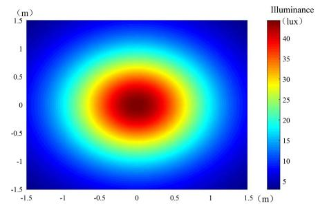
**Figure 1.** Illumination distribution of LED lamp.
