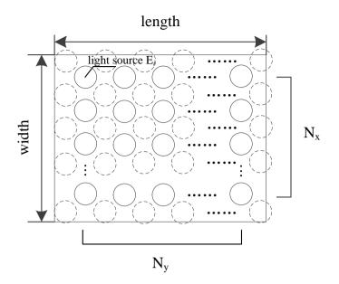
Figure 3. Distribution of light source displacement in agricultural greenhouse.
