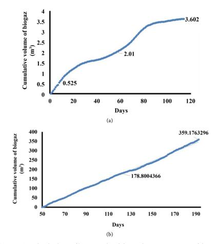
**Figure 2.** Cumulated volume of biogas produced during the monitoring time of the experimental (a) and pilot (b) digesters.
