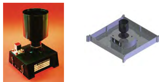
Fig 8 Star Sensor KM 1301 and its integration into the tray structure
