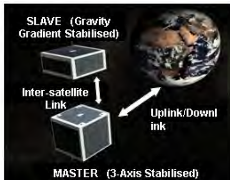
Fig 4 JAESat Communication Concept
