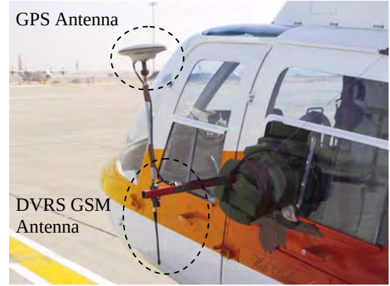
Fig. 1 System installation for the helicopter test
