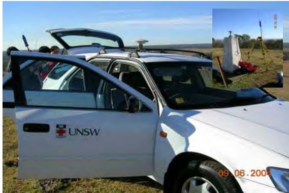
Fig. 5 A reference station and a rover
