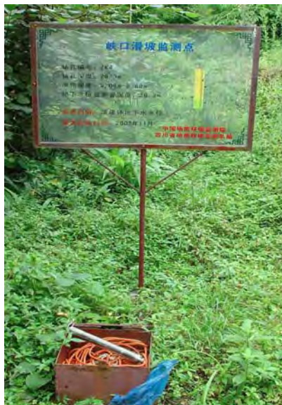
Fig. 6 Underground water level monitoring point
