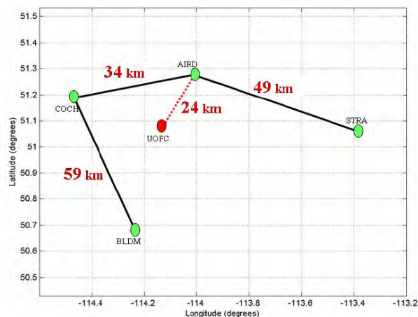
Fig. 2 Network configuration for the correction-based multiple reference station approach with UOFC as the rover
