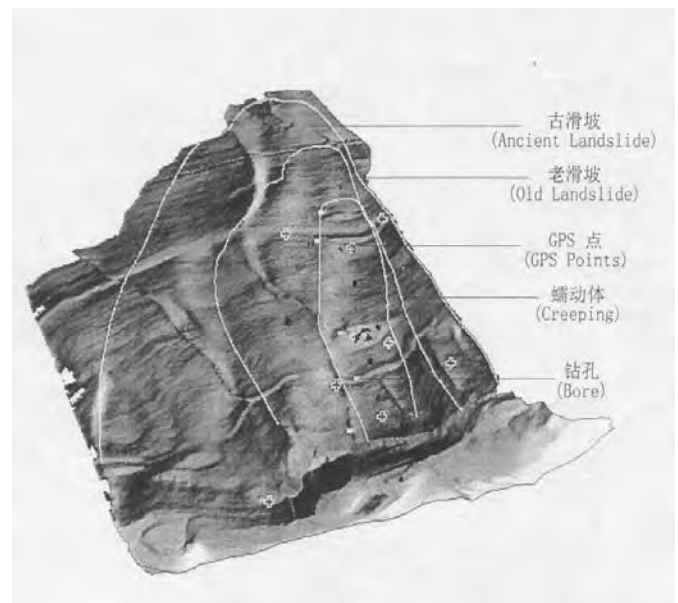
Fig. 1 Sliding mass at the Xiakou landslide 2.1 Reference Frames
