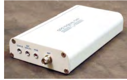
Fig.2 Picture of the GPS Signal Tap
