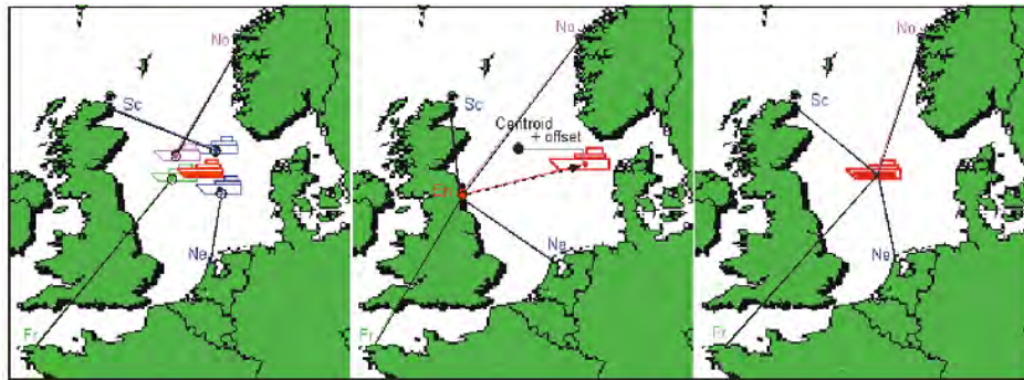
Fig. 3 The positioning methods using multi-DGPS references
