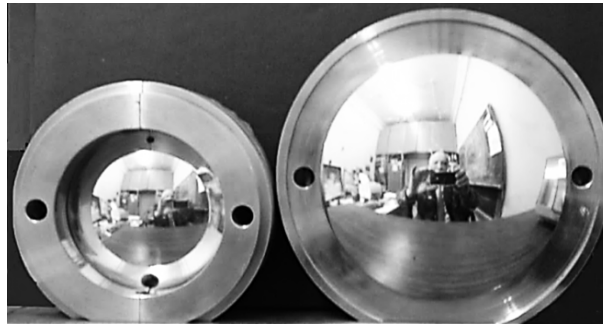
Figure 7. Prototypes of steel acoustical lenses for frequencies F = 3.5 MHz (left image) and F = 1.5 MHz (right image).
