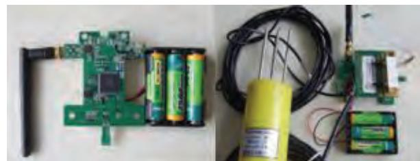
**Figure 1.** The NPUnode and equipped sensors.
