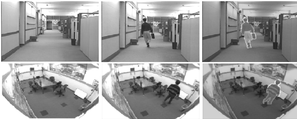
Figure 3. Detected foregrounds for indoor circumstances. The first column is the first frame of the sequences, the second column is the current frames (67th, and 300th, from top to bottom, respectively), and the third column is the detected foreground masks with light grey pixels superimposed on the original image
