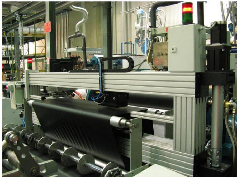
**Figure 26.** Radiometric profile meter—head with traverse, MM-06 type [26].
