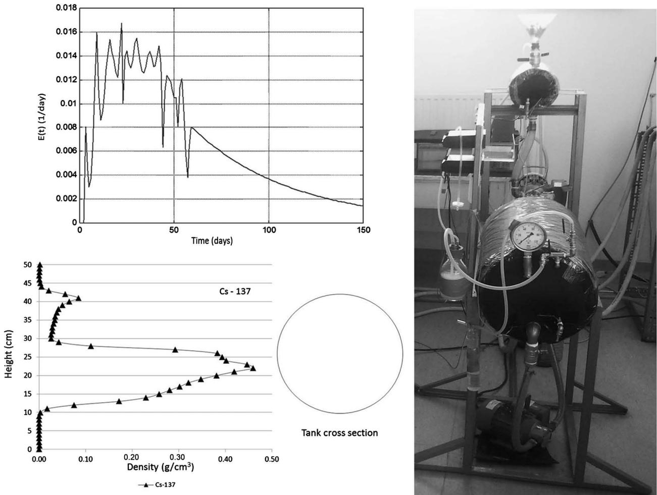
**Figure 3.** Comparison of experimental and model RTD results and scheme of scanning measurement and distribution of the density inside the fermenter [12].
