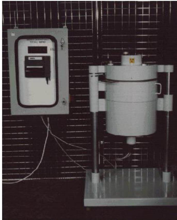
**Figure 9.** MPKF radiometric ash meter [13].
