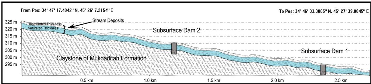
Figure 11. Longitudinal section along Isayi stream, illustrating location of the suggested subsurface dams with the stream deposits.
