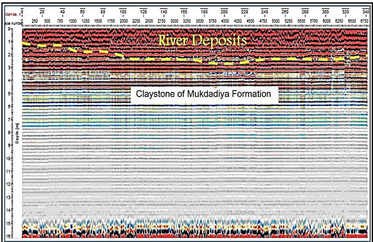
Figure 5. Radar section of the profile NO.2.
