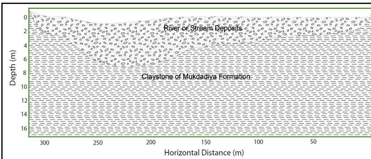
Figure 3. Geologic cross section for the proposed subsurface dam's selected site location.
