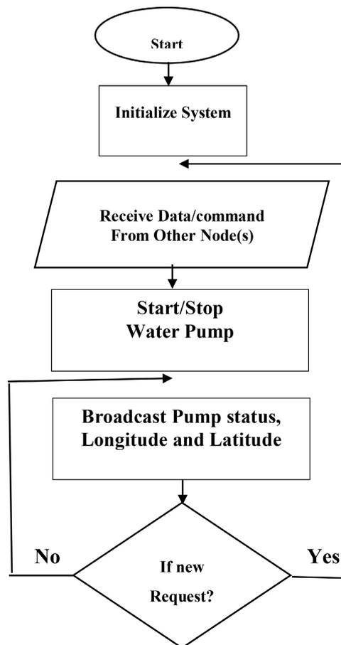
Figure 9. Actuator Node flowchart.
