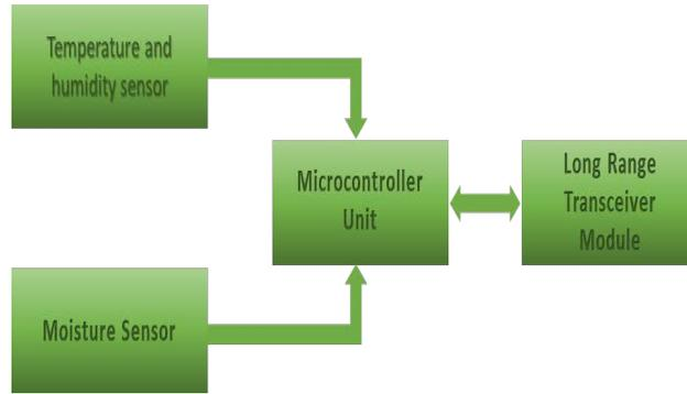
Figure 10. Sensor node architecture.
