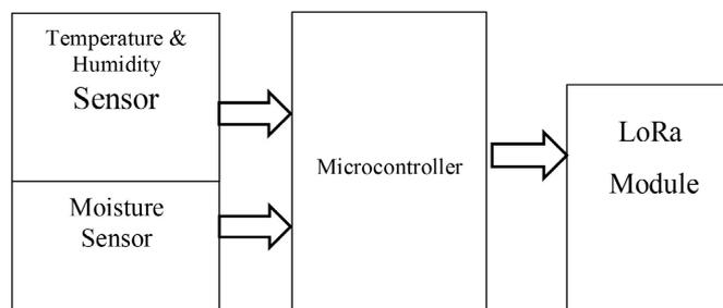
**Figure 2.** Smart agriculture sensor node gateway.
