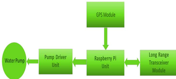
Figure 11. Actuator node architecture.
