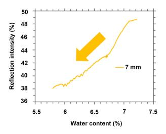
**Figure 6.** Reflection intensity from the concrete of 7 mm thickness.
