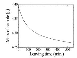
Figure 2. Mass change of concrete by leaving.
