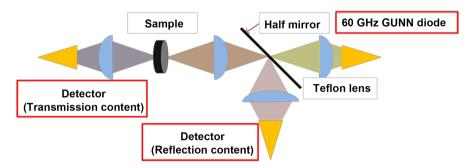
Figure 3. The optical schematic system of THz transmittance and reflection measurement.
