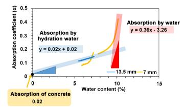
Figure 5. Relationship between thickness and sensitivity.
