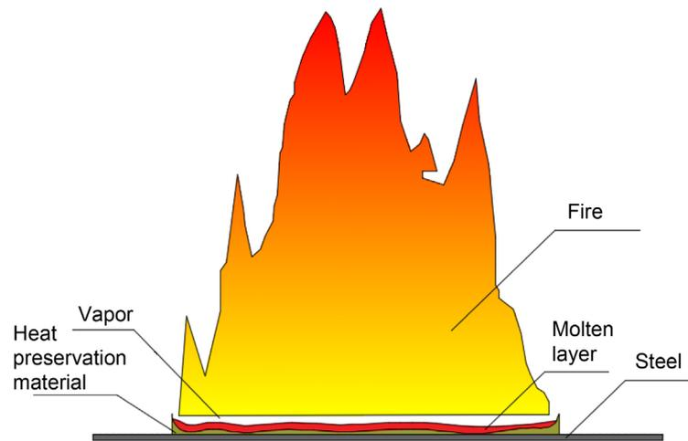
**Figure 1.** Schematic diagram of thermal insulation material combustion.
